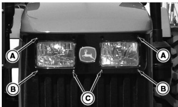
A—Headlight adjusting screws (2 pieces) C—Headlight adjusting screws (2 pieces) B—Headlight adjusting screws (2 pieces)
