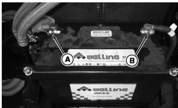
A—Positive (+) battery terminal B—Negative (-) battery terminal
