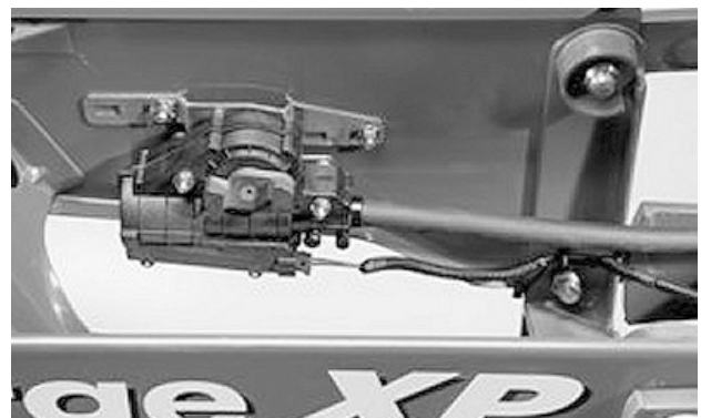
A67674—UN—11JUN10 Cuplaj RowCommand™ Pro-Shaft
