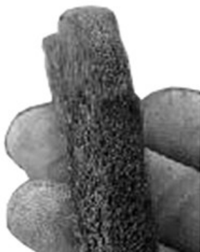
A100144—UN—21MAR18 Desgaste lateral irregular
