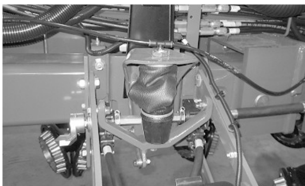
Resort pneumatic rulat necorespunzător
