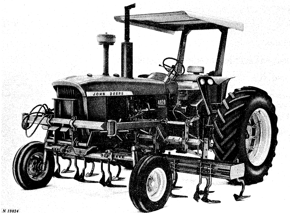
John Deere A20 Beet-Bean-Vegetable Cultivator on 4020 Row-Crop Tractor
