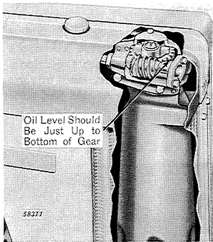
Steering Gear Oil Level (Manual Steering)
