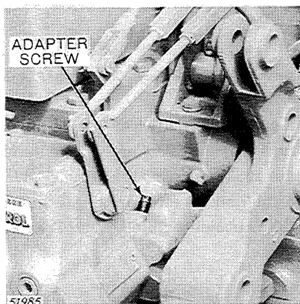
Single- or Double-Acting Remote Cylinder Adapter Screw on Dual Valve Housing
