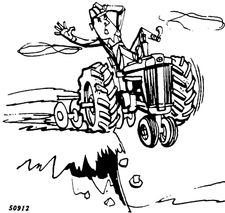
Never Drive Too Close to Ditches
