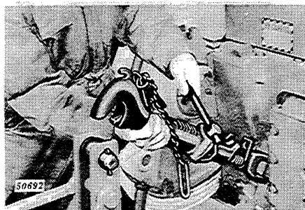
Attaching Upper Link to Implement Mast
