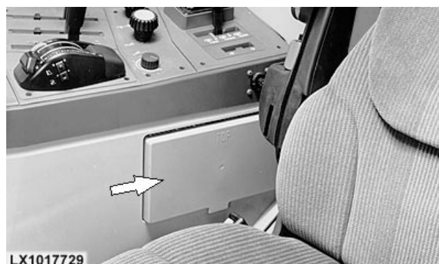
Fuses (tractors with cab)
