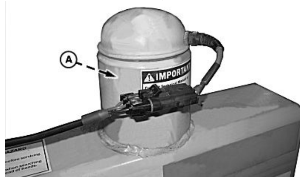
Incorporated Wheel Angle Sensor
