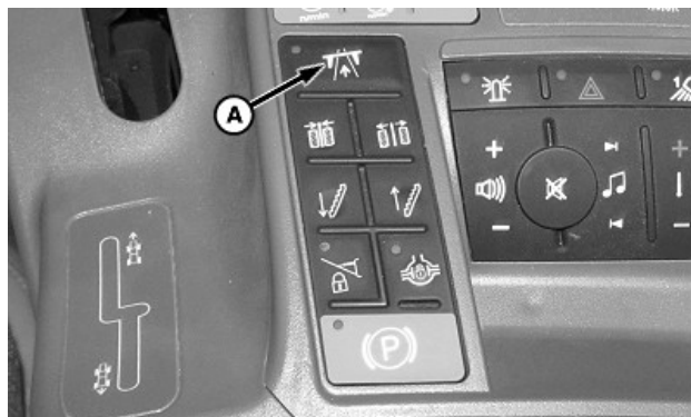
A—Transport Lock Switch
