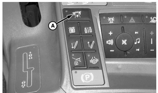
A—Transport Lock Switch
