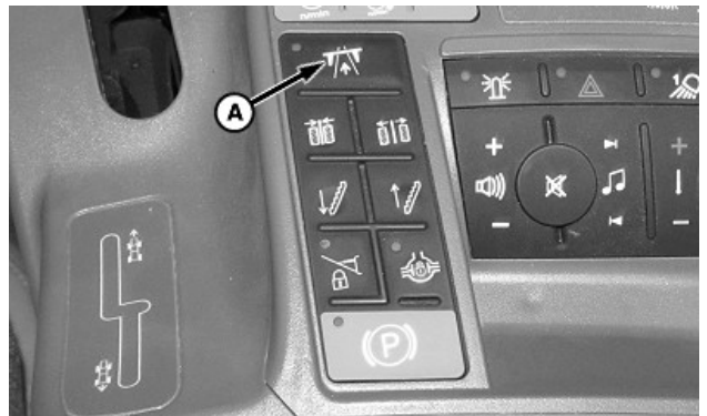
A—Transport Lock Switch
