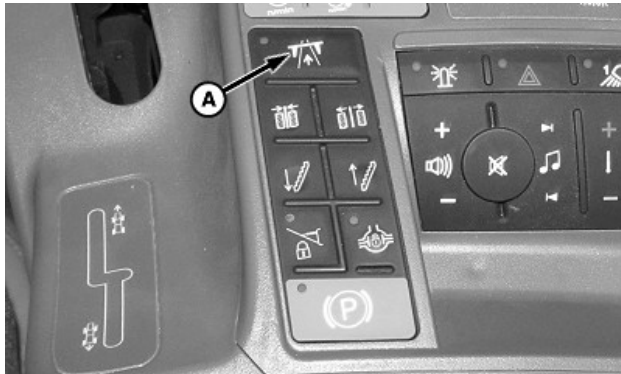
A—Transport Lock Switch
