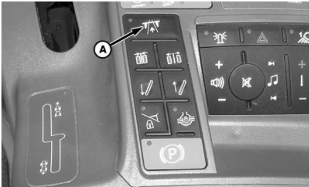
A—Transport Lock Switch
