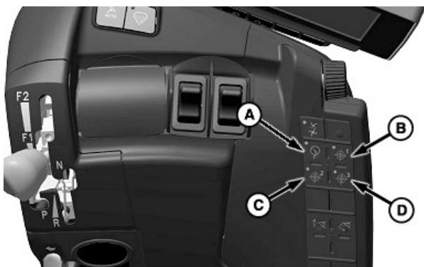
A—Manual Rate Selection Switch B—Preset Rate 1 Selection Switch C—Preset Rate 2 Selection Switch D—Preset Rate 3 Selection Switch
