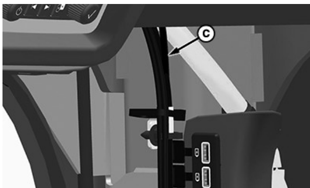
N160162—UN—06JAN22 Radio Power/Ground Cable behind Rear Corner Post Cover
