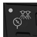
Nozzle Pressure Control
