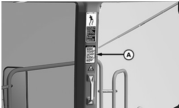
A—Engine Start/Idle Decal
