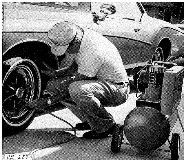
Using the sprayer — inflating tires
