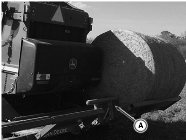
A—Right-hand slider position (Bale on right-hand wing)
