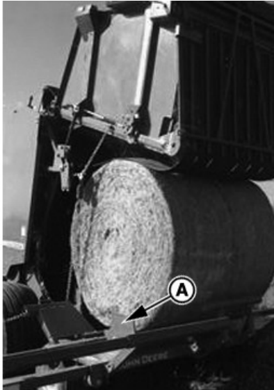
A—Left-hand slider position (Bale in middle of cart)
