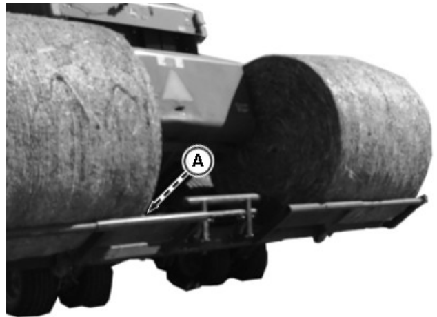
A—Third Position of the Slider (When baler gate closed)
