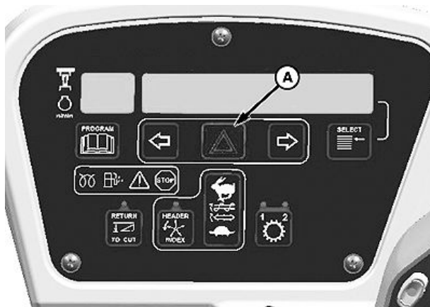
Hazard Light Switch
