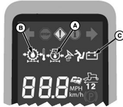
A—Oil Pressure Lamp B—Hydrostatic Pressure Lamp
