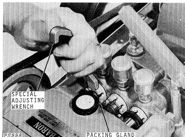
Adjusting Plunger Seals on A25 Washer
