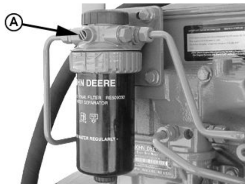
Final Fuel Filter Bleed Vent Screw
