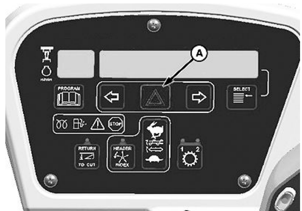
Hazard Light Switch
