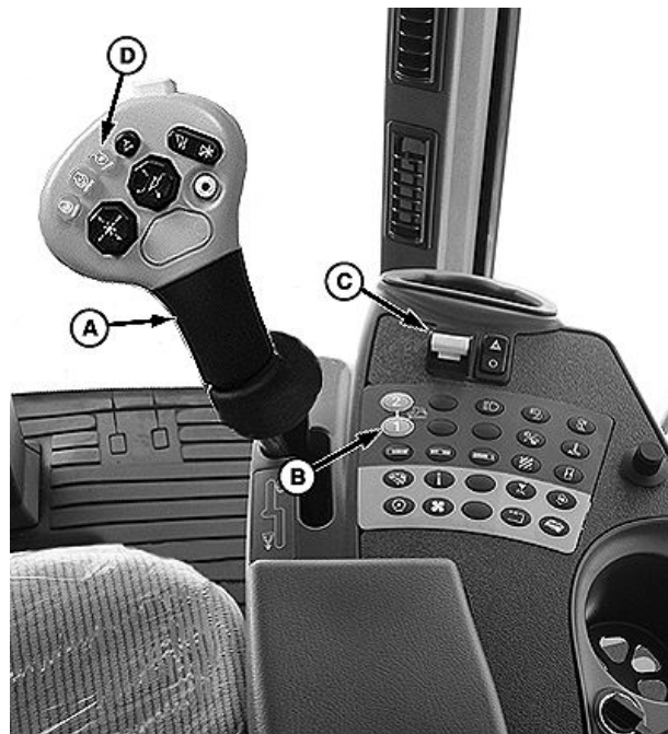
A—Multifunction Control Handle B—Low Speed Switch (1)
