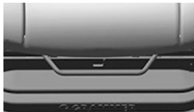
Positionsregulering fremad/bagud - Select
