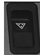
Trailing Lights Switch
