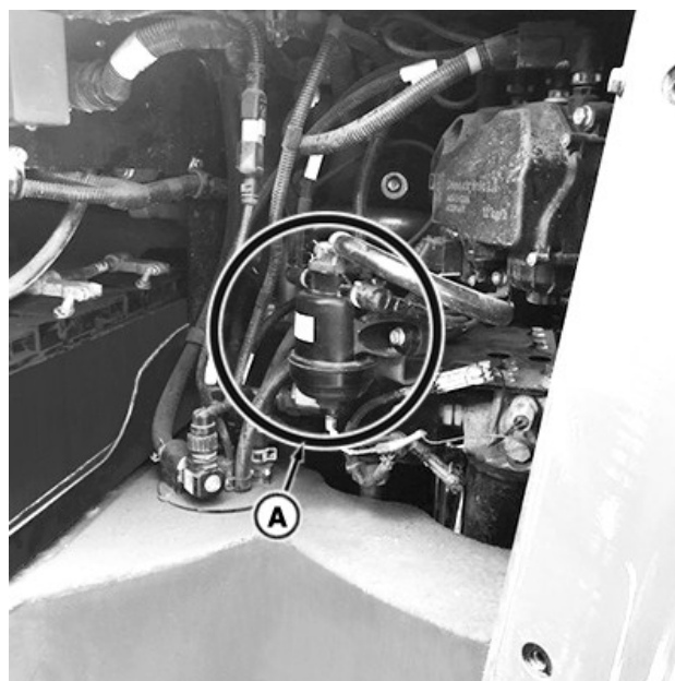
The DEF in-line filter (A) is inside the battery compartment.
