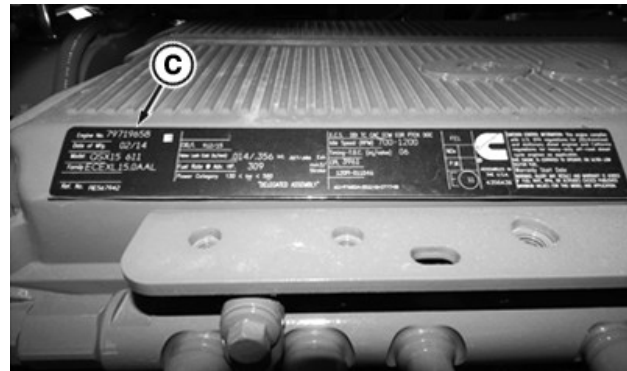
Engine Serial Number Plate (C) is on the Left-Hand Side of the Engine Valve Cover
