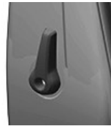
RXA0167342—UN—03APR19 Control de ajuste lumbar - Select
