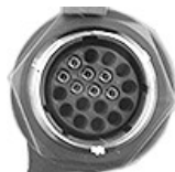
RXA0167988—UN—17MAY19 Conector del monitor GreenStar™
