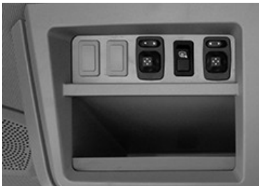
RXA0168462—UN—31MAY19 Electric Mirror Controls Example
