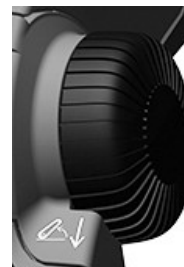
RXA0168025—UN—17MAY19 Hitch Depth Adjust Dial
