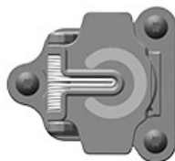
RXA0188747—UN—07MAR23 Implement Ethernet Connector
