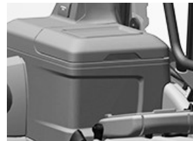
RXA0167977—UN—17MAY19 Refrigerator and Cool/Storage Box Example
