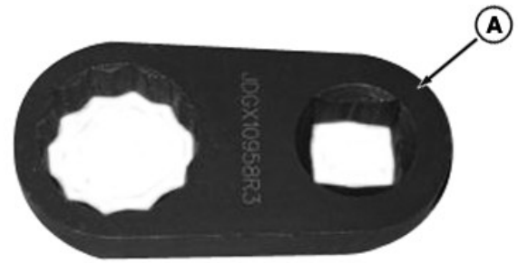
JDG10958 Wheel Weight Holding Wrench
