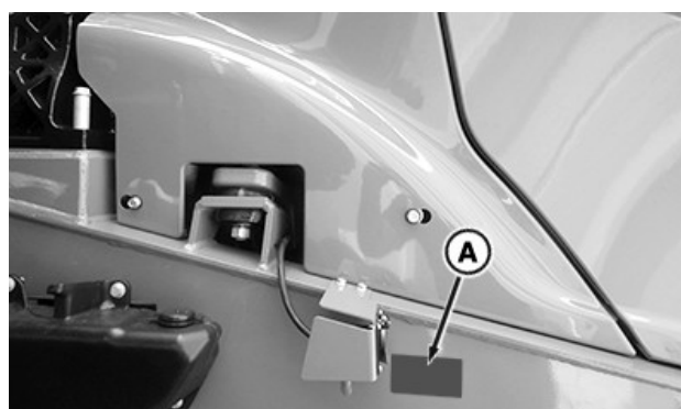
A—Engine Heater Label (right-hand side of tractor near heater connector)
