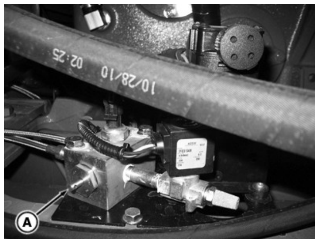
Vent Valve-Above Suspension Axle
