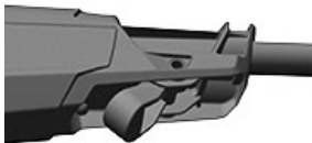
RXA0167461—UN—12APR19 Manual Telescoping Lock Lever
