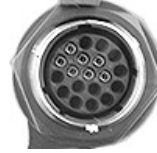
RXA0167988—UN—17MAY19 Conector para el monitor GreenStar
