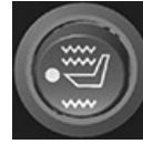
RXA0173801—UN—14JAN20 Vent/Heat Intensity Control - Ultimate
