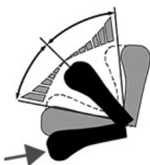
RXA0173491—UN—02JAN20 Position flottante
