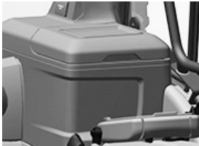
RXA0167977—UN—17MAY19 Refrigerator and Cool/Storage Box Example
