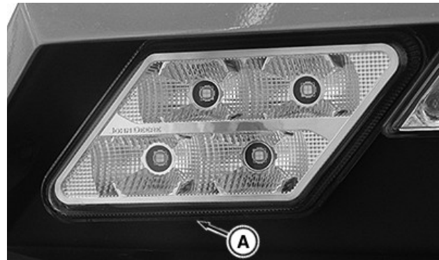
RXA0172759—UN—03DEC19 Cab Roof Light—LED Light Option Shown
