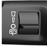
RXA0167459—UN—12APR19 Right-Hand/Rear Wiper Speed/Washer Lever
