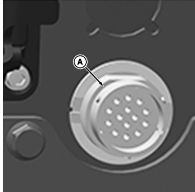
AutoLoad™ Harness Connector Outlet is Above the SCV Stack
