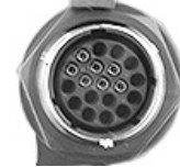
RXA0167988—UN—17MAY19 Conector para el monitor GreenStar
