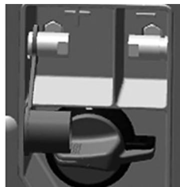
The battery jumper terminal posts are located near the tractor steps.
