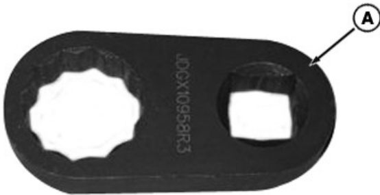
JDG10958 Wheel Weight Holding Wrench
