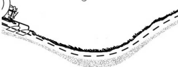
In rolling terrain, high value causes less depth variation.
