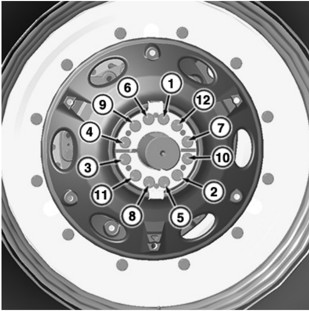
Torque sequence: Double-flat heavy-duty drive wheel hub assembly
