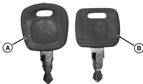
Immobilizer Key Compared To Standard John Deere Key
