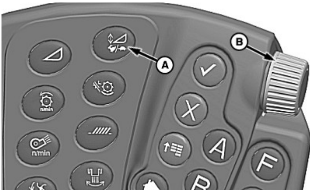
A—Feeder House Rate/Sensitivity Adjust Switch B—Selection Dial
