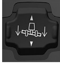
H116348—UN—19DEC16 Header Raise/Lower Switch (Style B)
