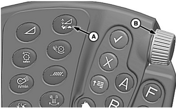
A—Feeder House Rate/Sensitivity Adjust Switch B—Selection Dial
