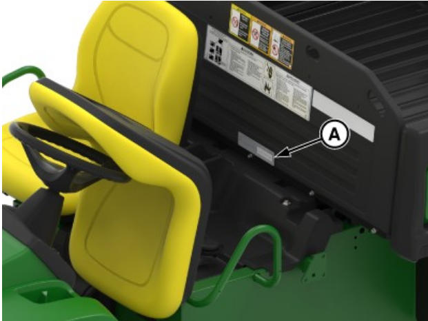
Label is installed on cab behind driver seat belt assembly
