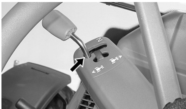
Park Lock Engaged on AutoPowr™/IVT™
