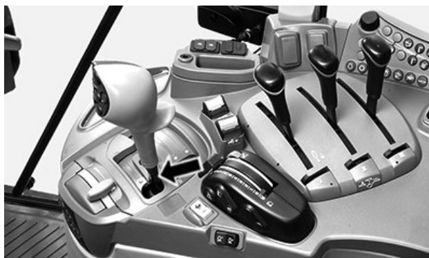
Park Lock Engaged on PowrQuad™/AutoQuad™
