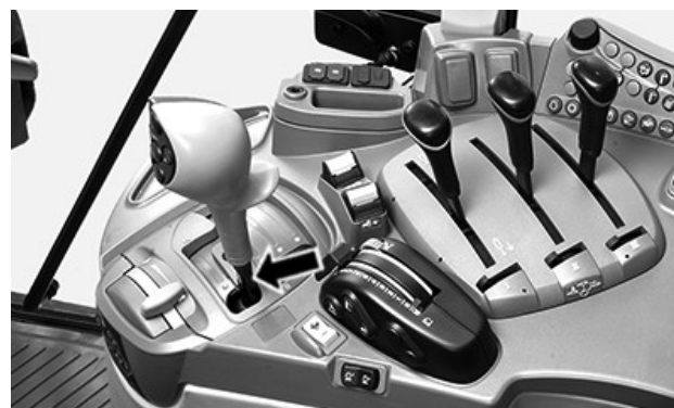
Park Lock Engaged on PowrQuad™/AutoQuad™
