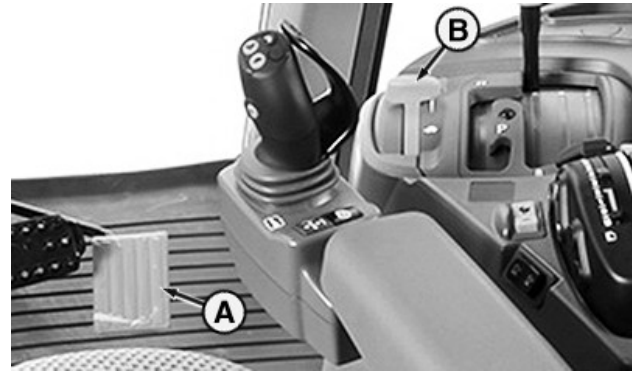
A—Speed Control Pedal B—Hand Throttle
