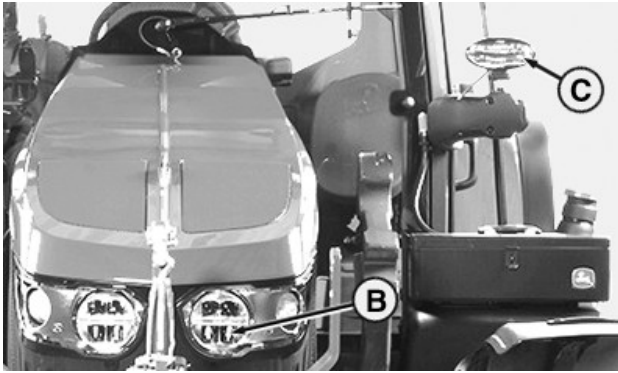
B —High/Low-Headlights on the Hood C —High/Low-Beam Headlights on Cab Frame (optional)
