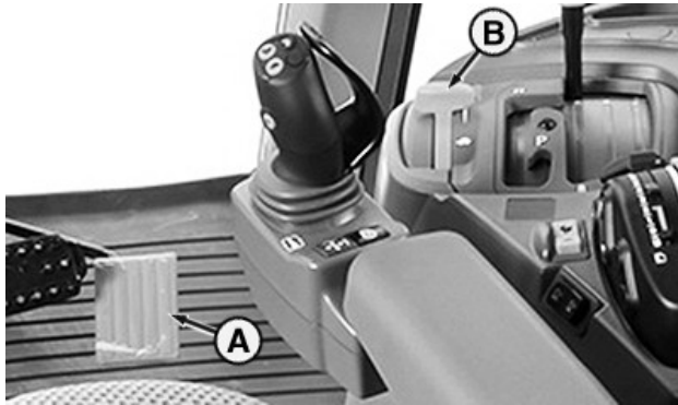
A—Speed Control Pedal B—Hand Throttle
