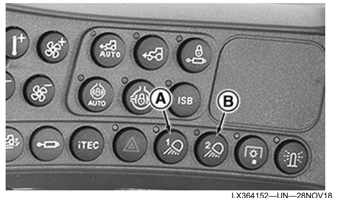
A—Worklight 1 ON/OFF B—Worklight 2 ON/OFF
