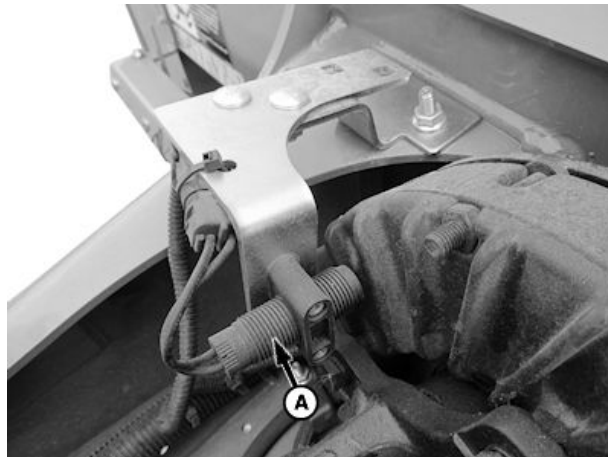
PTO Sensor (540 rpm) Shown
