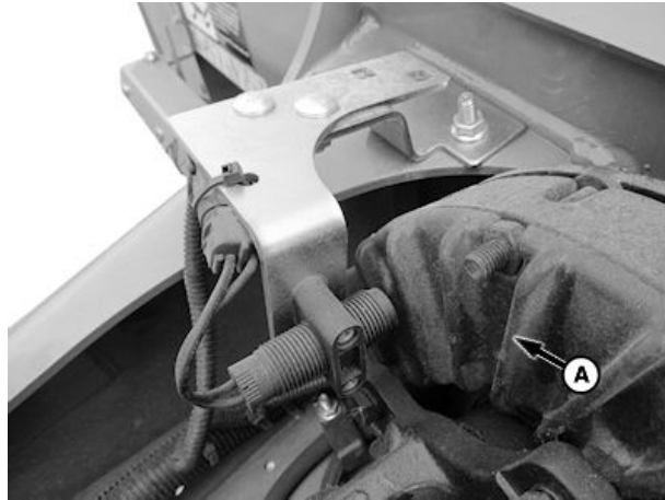
PTO Sensor (540 rpm) Shown
