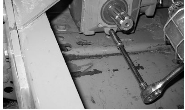
Removing Drain Plug
