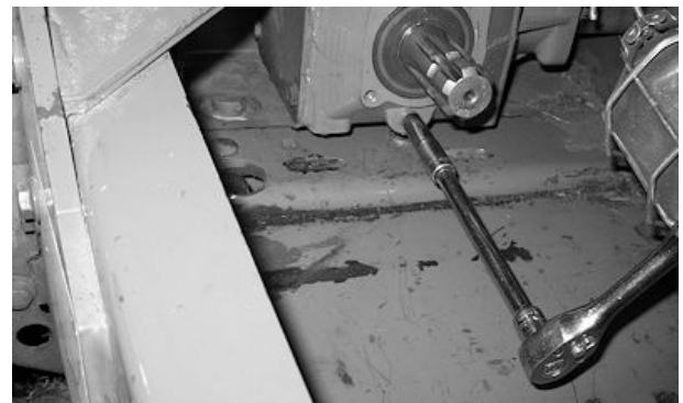
Removing Drain Plug
