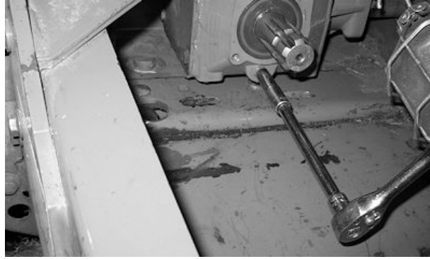
Removing Drain Plug
