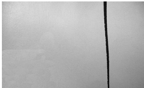
Smooth Cut From Sharp Knife
