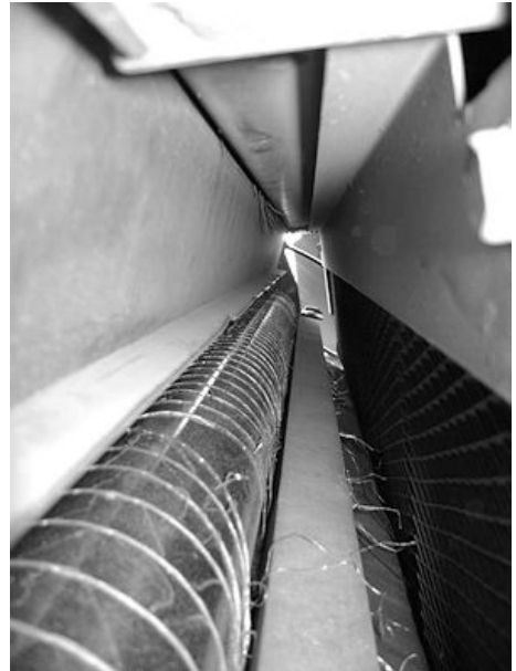
Net Material Against Steel Roll
