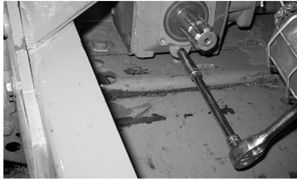
Removing Drain Plug
