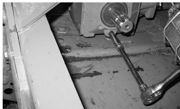
Removing Drain Plug
