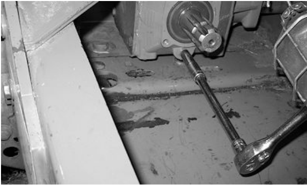
Removing Drain Plug
