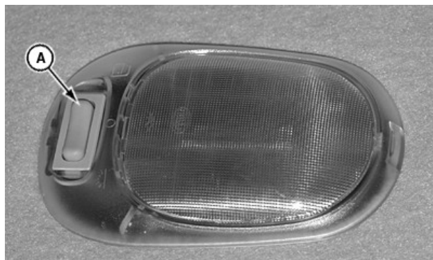
A—Dome Light Switch
