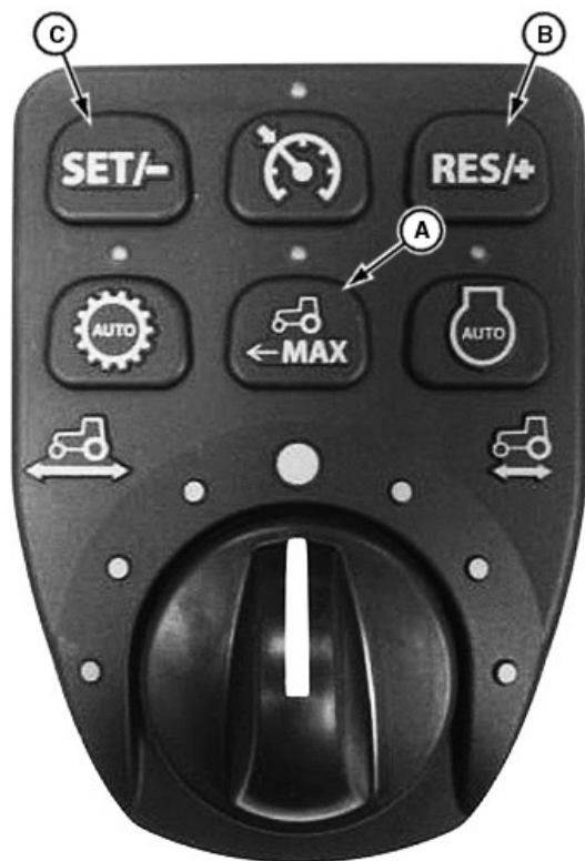
A—Interruptor SpeedMatch B—Interruptor RES/+ C—Interruptor SET/-
